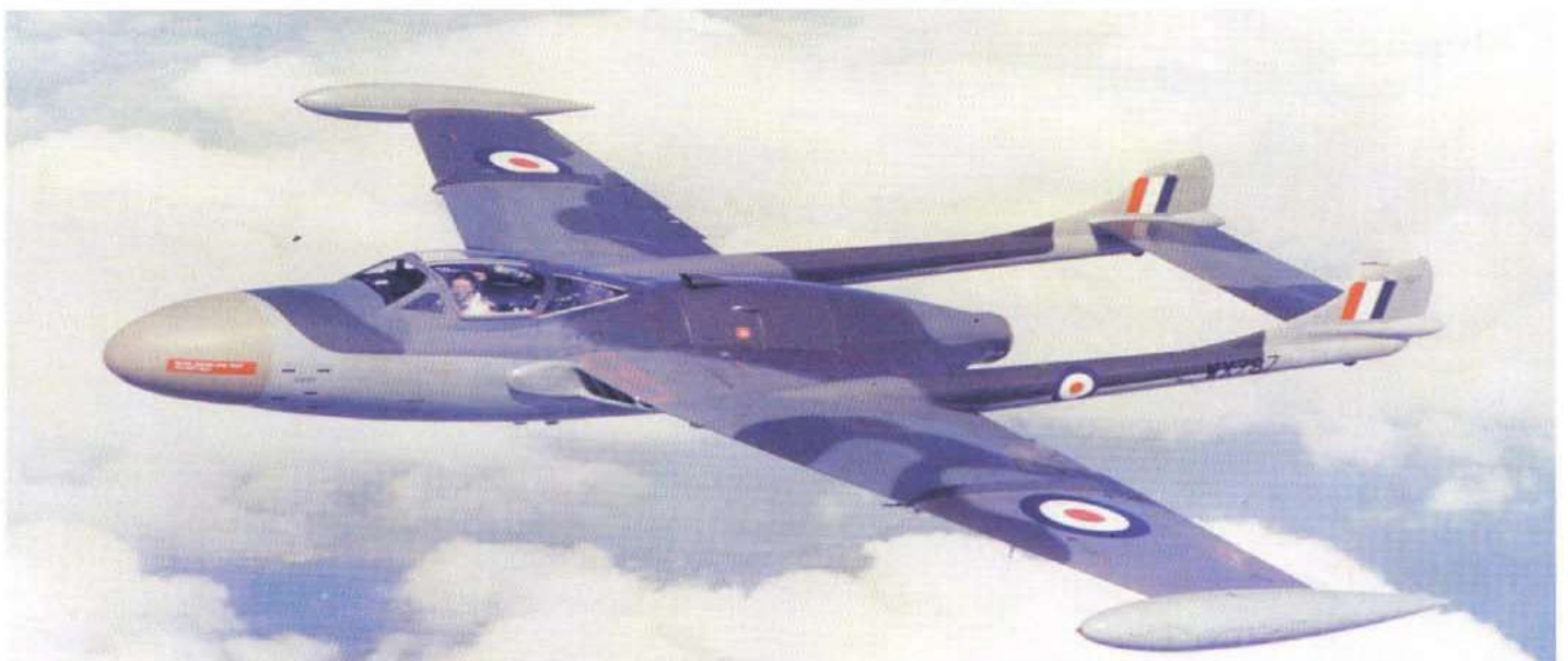
Left: Displaying the markings of black and white horizontal triangles this Venom NF.3 WX840:L, was in use with No. 141 Squadron in 1956. (MAP) Below: Venom NF.3 WX787 was used for manufacturers trials at A&AEE. The deletion of the outer sections of the tailplane can be seen along with the much improved clear view cockpit canopy.
