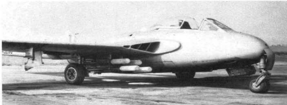
Another view of FB.1 WE258 while conducting rocket projectile firing from Boscombe Down in 1952. The two-tier R/Ps have concrete heads, used for training purposes.
