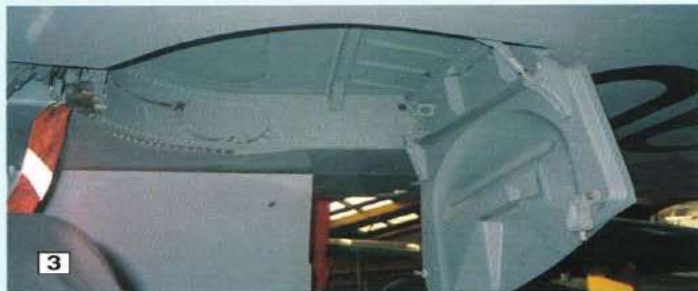
1. Starboard main undercarriage leg on Venom FAW.22 WW217 2. Venom NF.3 WX905 canopy and stencil detail. 3. Undercarriage wheel well of the same NF.3 including the undercarriage door. 4. The rear of the left hand boom acorn shape on the NF.3 which contained the navigation light. 5. The fins and rudders of the Venom NF.3 WX905 preserved at Newark.
