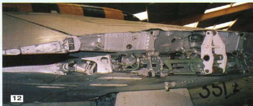
12. The complicated interior of the wing folding mechanism on th Venom FAW.22 can be see in this picture. 13. The nose wheel of the FAW.22 which is worth comparing with the NF.3 above. (Allcolour pictures taken at the Newark Air Museum)
