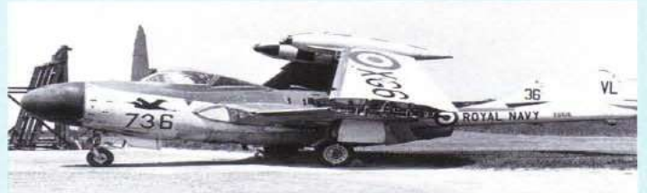
Above: FAW.22 XG682. The 'nib' over the arrester hook shows up plainly. Below: FAW.21 XG616: 736-VL of 766 Squadron. (APN)
