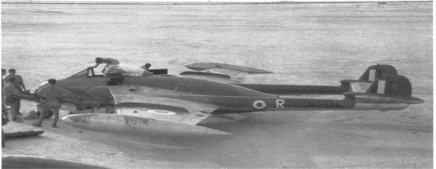
Ground crew of No. 8 Squadron contemplate problems with WR561:R at Sharjah in early 1958. The gun bay doors are off so that was probably the root of the problem. Note the main runway in the background made from compressed sand and responsible for the sand-blasted appearance of the squadron's aircraft.
