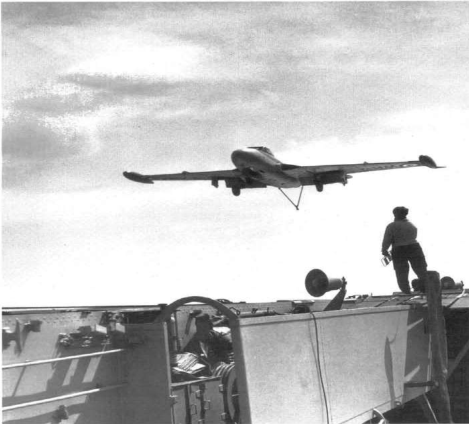
Above: Approaching to land on Ark Royal , Sea Venom FAW.21 WM574 was engaged in experimental blown flap trials in April 1956. It later served at RAE Farnborough and the Empire Test Pilots School coded 18. Below: No. 891 Squadron on board Bulwark in July 1955. FAW.21 WW146:438-O is in the foreground showing the squadron's 'Kon Tiki' crest.
