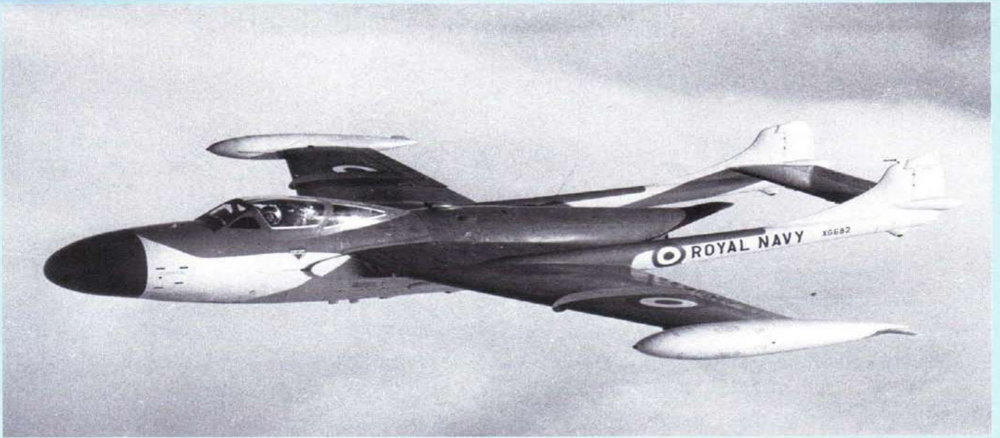
Above: FAW.22 XG682. The 'nib' over the arrester hook shows up plainly. Below: FAW.21 XG616: 736-VL of 766 Squadron. (APN)
