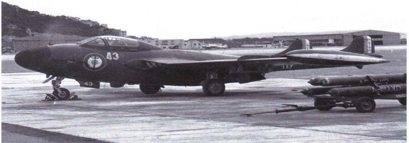
Above: Aquilon 201 of Flotille 11F which formed at Hyeres in mid-1955. Below: A SNCASE-built Sea Venom built under licence and known as the Aquilon (North Wind) for the French Aeronavale. They were mostly finished in a midnight semi-gloss blue.
