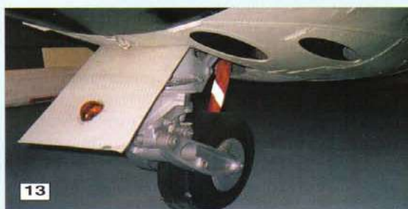
12. The complicated interior of the wing folding mechanism on th Venom FAW.22 can be see in this picture. 13. The nose wheel of the FAW.22 which is worth comparing with the NF.3 above. (Allcolour pictures taken at the Newark Air Museum)
