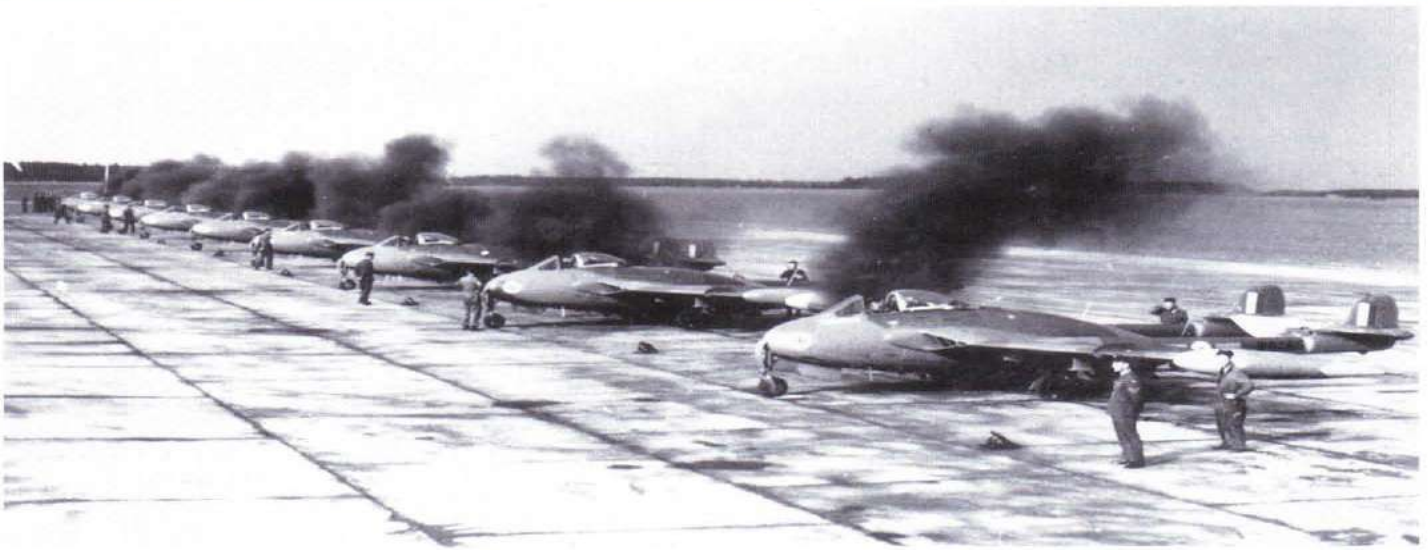
It looks as if all of these Venom FB.4s of No. 5 Squadron are on fire. The cloud of black smoke caused by the starter cartridges did tend to frighten the uninitiated. The picture was taken in 1956 and all aircraft displayed the squadron badge on the nose. The aircraft in the foreground is WR485. (MAP)
