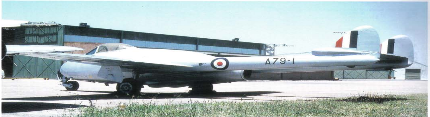
One way to try and improve performance of the Australian F.30 was to move the 'elephant ears' under the fuselage and many aircraft were so converted, including the first F.30 built A79-1, seen here in 1982. (MAP)
