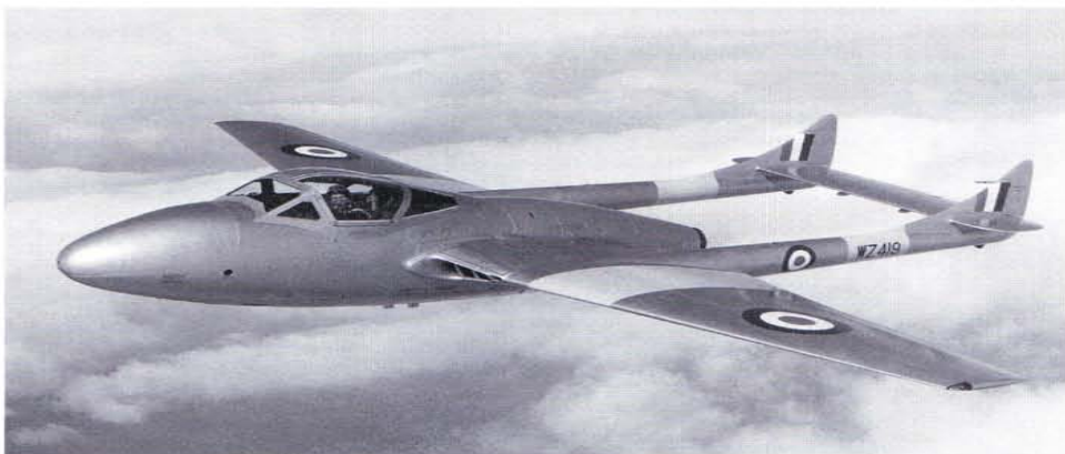
Above: The prototype Vampire Trainer in Class B markings G-5-7 and still in its overall silver finish. First flight was at Christchurch on 15 November 1950 with John Wilson at the controls. There were no problems with the flying characteristics and the T.11 went straight into production. (BAe) Right: The sixth T.11 off the production line WZ419, was used by de Havilland to test the new canopy and other improvements, including the installation of ejection seats. It eventually became 7420M. (BAe)
