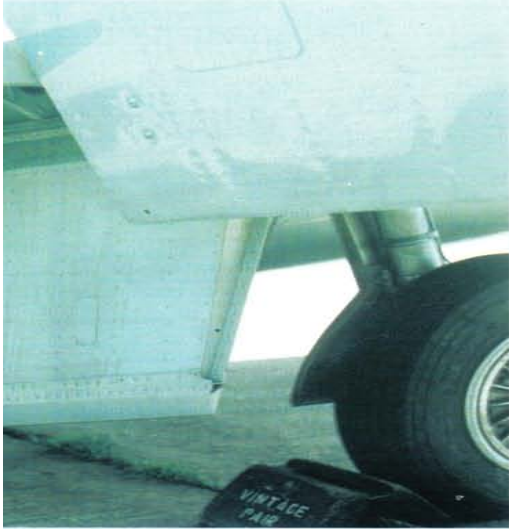
3. Good detail view of flaps in the down position on the Vampire FB.5. High right is the airbrake. 4. Vampire FB.5 ailerons, with balance tab, air brake and flaps. 5. The familiar tailplane of a Vampire FB.5 showing the 'acorn' or 'bullet' fairing the boom to the tail. The small rubber buffers under the rear of the boom are to prevent damage if the aircraft is rotated too smartly, or after landing when the nose should be kept high to present the maximum airframe area to assist with aerodynamic braking.
