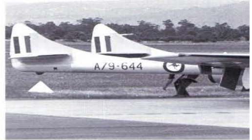
The RAAF used a simple coding system, using the last two digits of the serial number. Anticollision markings were applied on the upper nose section and dorsal fins. A79-644 was photographed in 1968. (MAP)
