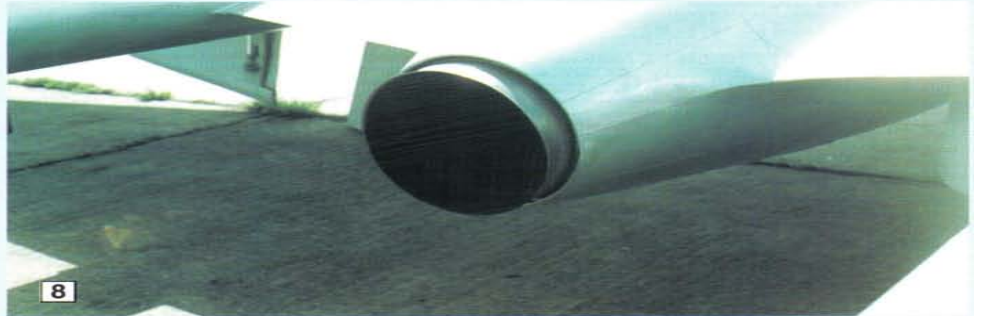
6. and 7. Two views of the Vampire FB.5's main undercarriage leg, bay, doors and area. 8. Jet pipe exhaust at the rear of the fuselage pod.
