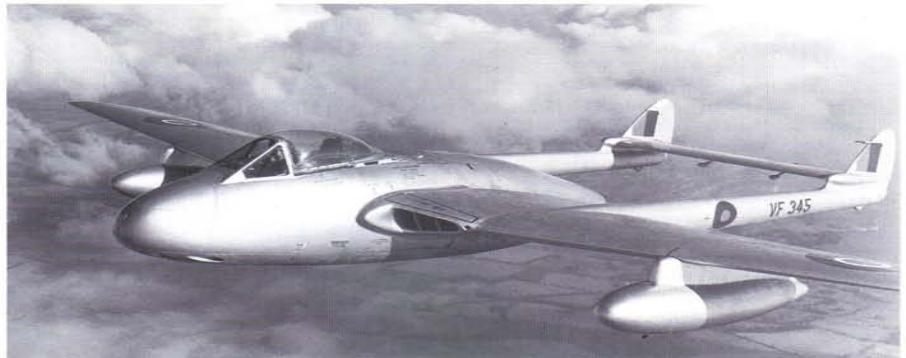
Above: Vampire F.3 VF345 showing off the new pylon-mounted drop tanks. The small protrusions under the rear of the tail booms were to offset any damage caused by spirited pilots rotating too sharply on take-off! It joined No. 73 Squadron at Malta but overshot when landing at Bergamo, Italy, on 27 October 1949. (BAe) Below: VF344:ZY-S, an F.3 of No. 247 Squadron before joining the RAuxAF where it served with Nos. 604, 614 and 608 Squadrons. (MAP)
