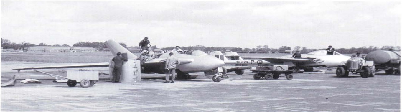
Above: Full of atmosphere, this interesting picture shows TG278 in its height record condition next to one of the DH.108s. Left: Vampire F.1 TG270 on the grass at Wolverhampton Airport after having the air intakes heavily modified to provide the Nene engine with more air. Compare the more sharply defined layout to the normal Vampire air intake. (Alec Brew, Boulton Paul Association)
