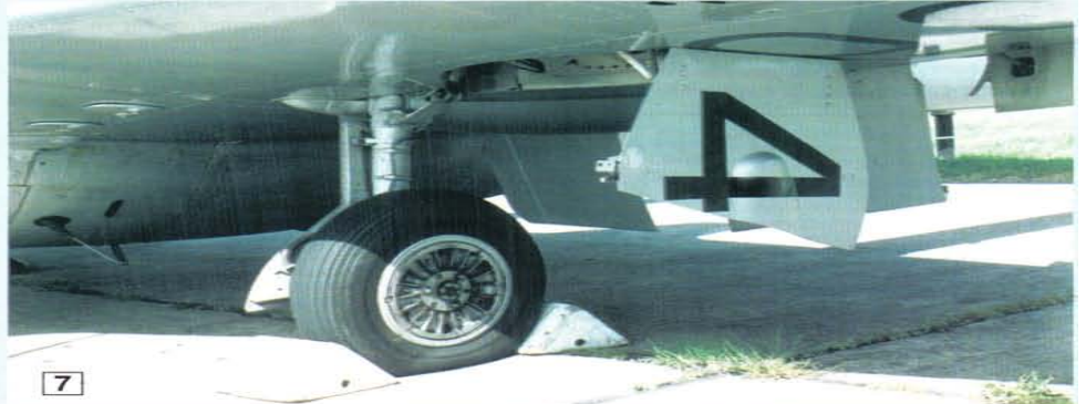
6. and 7. Two views of the Vampire FB.5's main undercarriage leg, bay, doors and area. 8. Jet pipe exhaust at the rear of the fuselage pod.
