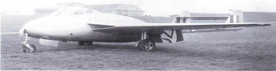
Above: Full of atmosphere, this interesting picture shows TG278 in its height record condition next to one of the DH.108s. Left: Vampire F.1 TG270 on the grass at Wolverhampton Airport after having the air intakes heavily modified to provide the Nene engine with more air. Compare the more sharply defined layout to the normal Vampire air intake. (Alec Brew, Boulton Paul Association)
